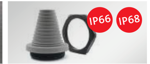
Cable entry grommets for screw-in assembly, M25 – M85, for cable diameters up to 70 mm KEL-DPF
