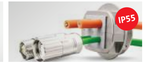
EMC Split cable gland for screw-on assembly with a locknut M32, M63 for cable diameters up to 35 mm
