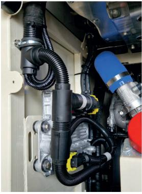
"We mainly use Harnessflex® NC conduit in various different sizes depending on the wire cluster size. We will also use their CTPA conduit on larger gauge or main power cables to allow it to be as flexible as possible, helping maintain mechanical reliability and fatigue life."
