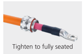
Tighten to fully seated 4. Tighten the pressure nut
