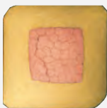
Micrograph of a square crimp
